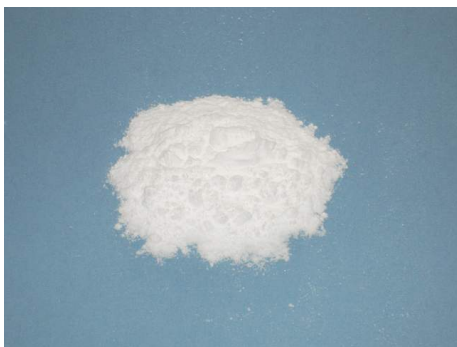
Crystals of potassium metabisulfite: the most common way to add sulfur dioxide to wine and must
