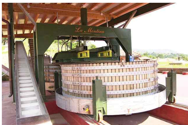
One of the Tenuta La Montina's Marmonier vertical presses
