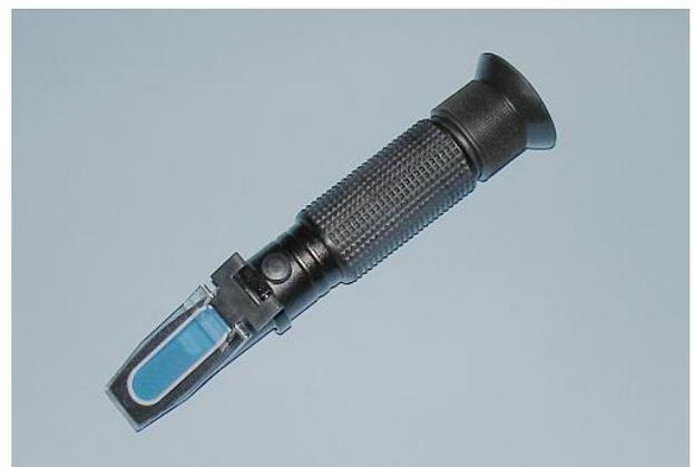
A portable refractometer
